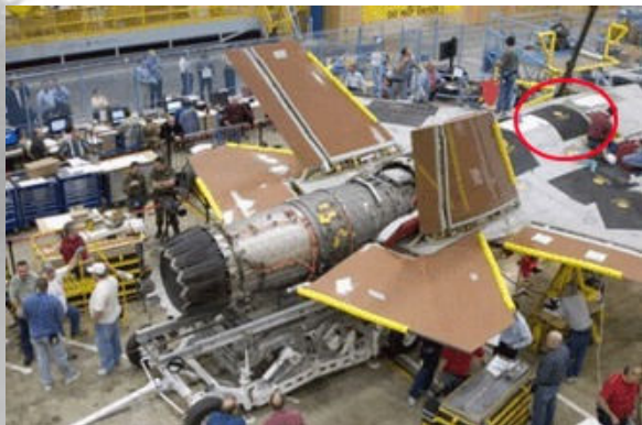
Plastic Reinforcements FOD Shield surface mat is used to protect the surfaces of the F35 Lightning II JSF (Joint Strike Fighter) from foreign objects
