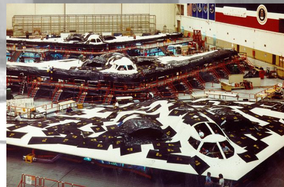
Plastic Reinforcements FOD Shield surface mat is used to protect the surfaces of the B2 Bomber from foreign objects
