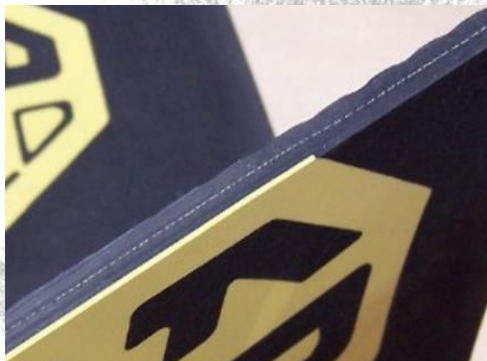
Edge View Showing Embedded Membrane
